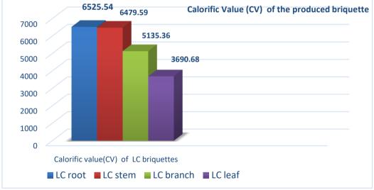
Figure 6: Calorific value (CV) of the produced LC briquette
