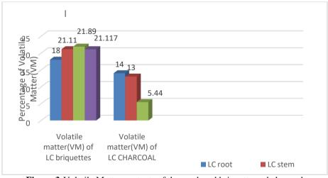
Figure 3: Volatile Matter contents of the produced briquette and charcoal
