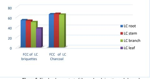
Figure 5: Fixed carbon content of the produce briquettes and charcoal
