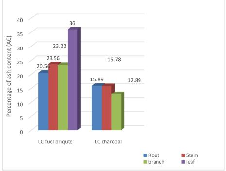
Figure 4: Ash contents of the produced briquette and charcoal
